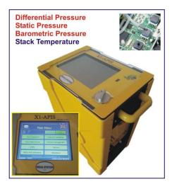
Thanks to the use of independent pressure sensors is possible to comply all the requirements of Table 3 (Performance Requirements), Table 4 (Performance Requirements during field measurements) and Table A.1 — Performance requirements for differential pressure-based flow measurement
